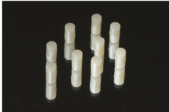
**Figure 3.** G-PMMA cylindrical samples.
