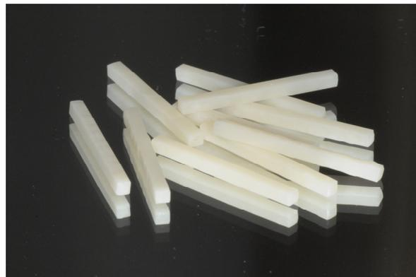
**Figure 1.** G-PMMA prismatic-shaped specimens after the finishing procedures.
