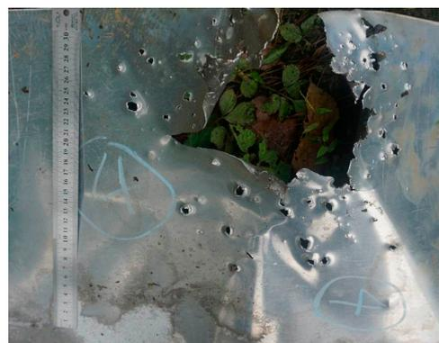
**Figure 11.** Typical damaged aluminum target plate.
