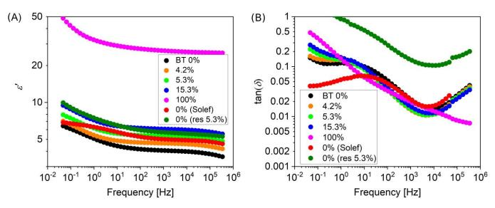
**Figure 2.** Frequency dependence of the dielectric constant (**A**) and loss tangent (**B**) of RAFT PVDF, PVDF-*g*-BT nanocomposites with the three different volume fractions of BT, the residual ungrafted PVDF extracted from the 5.3 vol% nanocomposite, the Solef PVDF, and the as-received BT nanoparticles, at 20  $^{\circ}$ C.
