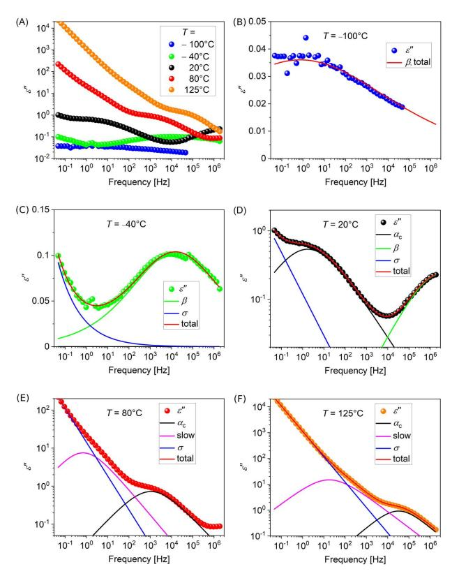
**Figure 3.** (**A**) Frequency dependence of the dielectric loss (imaginary part of permittivity) of RAFT PVDF at selected temperatures. (**B**–**F**): single spectra at each temperature, along with fitting curves related to the three relaxation processes as well as to the conductivity contribution. Blue curve: conductivity, green curve:  $\beta$  relaxation, black curve:  $\alpha_c$  relaxation, magenta curve: slow relaxation, red curve: overall fitting.
