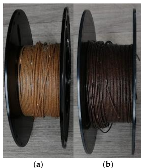
Figure 14. 3D printing filaments based on Colombian agro-industrial waste, (a) recycled PP/rice husk 10 wt.%, (b) recycled PP/cocoa bean shell 5 wt.%.
