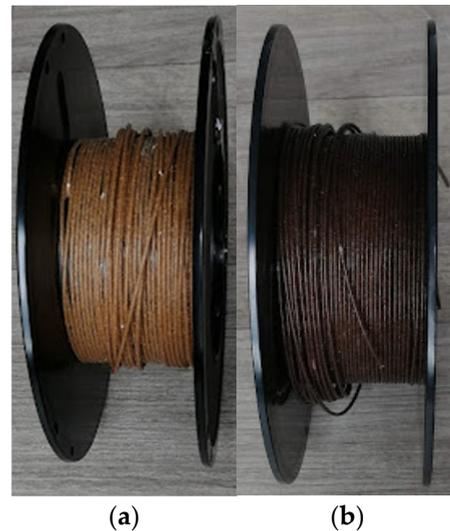
**Figure 14.** 3D printing filaments based on Colombian agro-industrial waste, (a) recycled PP/rice husk 10 wt.%, (b) recycled PP/cocoa bean shell 5 wt.%.
