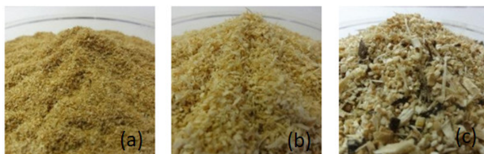
Figure 9. Different batches of sawdust used (a) (less than 0.7 mm), (b) (between 0.7 and 1.4 mm) and (c) (between 1.4 and 2.8 mm). From the project EcoPlast.
