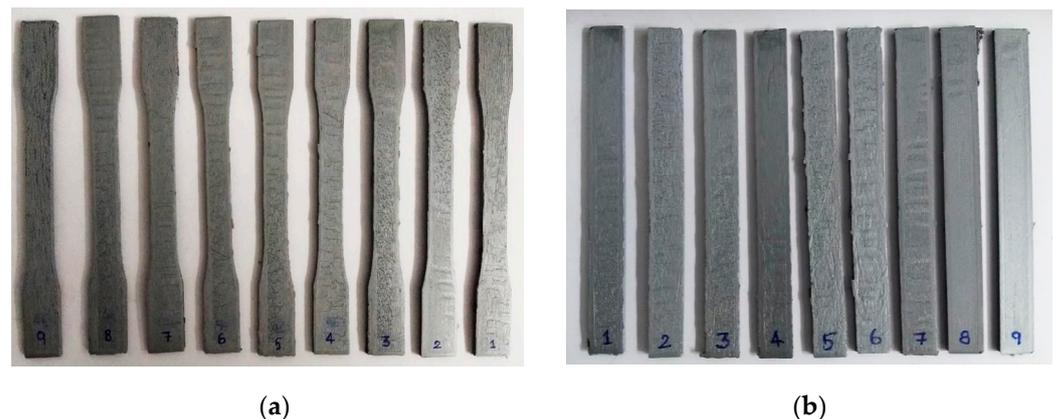
**Figure 5.** (a) Printed PLA-Al tensile specimens; (b) printed PLA-Al flexural test specimens.
