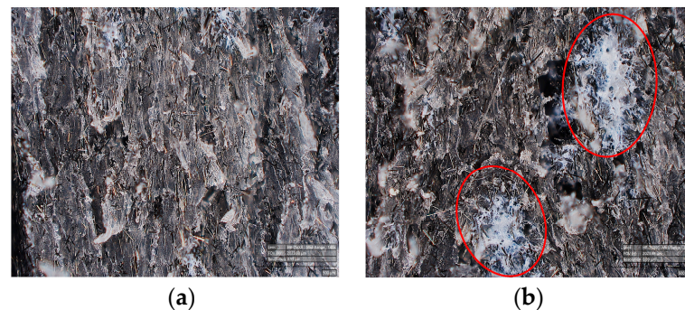
Figure 12. Micrographs of UHMWPE composites with LLDPE compatibilizers incorporated at (a) location I and (b) location II in the manufacturing process.
