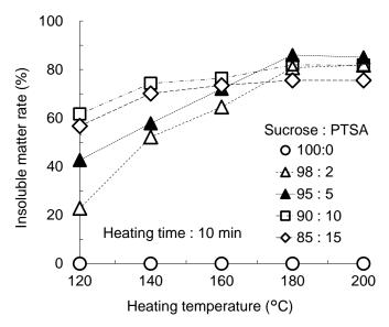
**Figure 3.** Effects of heating temperature on the insoluble matter rate of Suc-PTSA with different mixture ratios.
