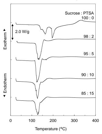
**Figure 1.** DSC curves of the dried mixtures of sucrose and *p*-toluenesulfonic acid (Suc-PTSA) with different mixture ratios.
