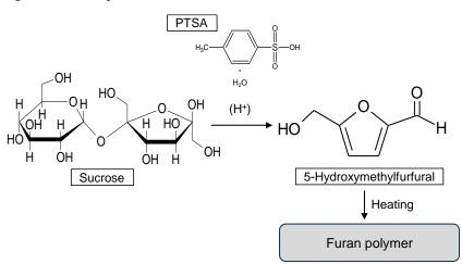
Figure 5. Expected reaction system for Suc-PTSA.
