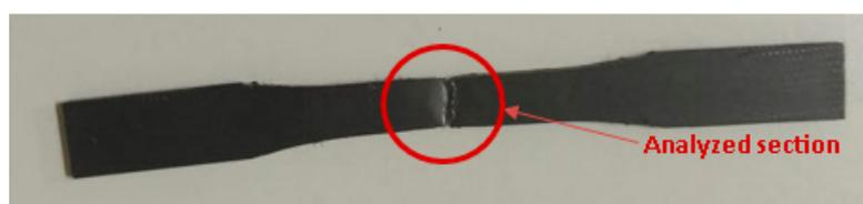
**Figure 3.** Cracked specimen.
