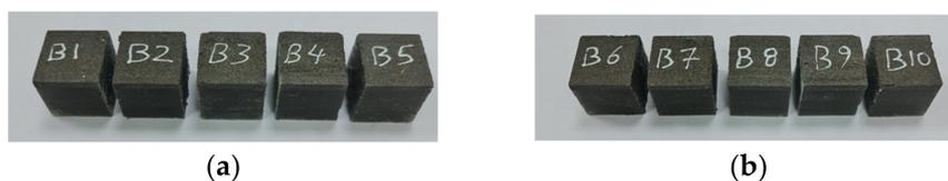
**Figure 6.** Compression test specimens (ASTM D3410). (a) untreated specimens (B1, B2, B3, B4 and B5) and (b) treated specimens with UVC (B6, B7, B8, B9 and B10).
