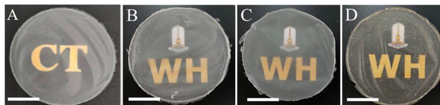
**Figure 1.** Macroscopic aspect of native CTC film (A) and CTC with 1.38% (B), 2.78% (C), and 4.14% (v/v) (D) glycerol. Note diameter of the plate is 9 cm and scale bars are 3 cm.
