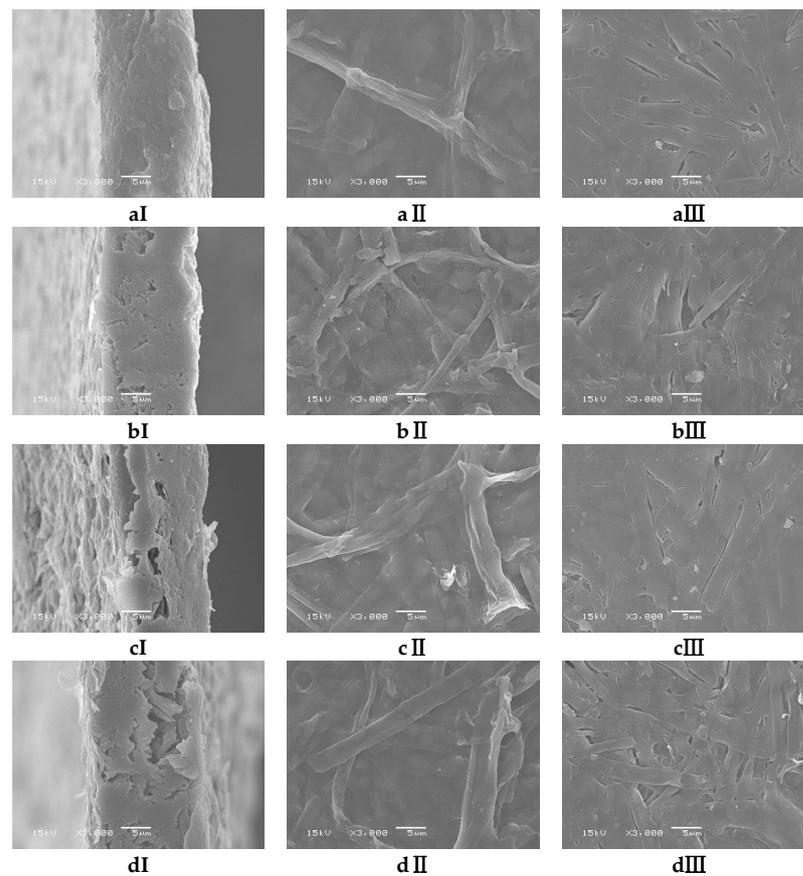
**Figure 2.** SEM micrographs of CTC films without (a) and with different glycerol contents of 1.38% (b), 2.78% (c) and 4.14% (*v/v*) (d); imaging of the cross-section (I), the top surface (II), and the side attached to petri dishes (III) with 3000 $\times$  magnification.
