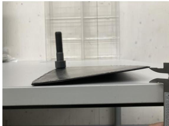
**Figure 5.** Warpage measurement of a consolidated plate.
