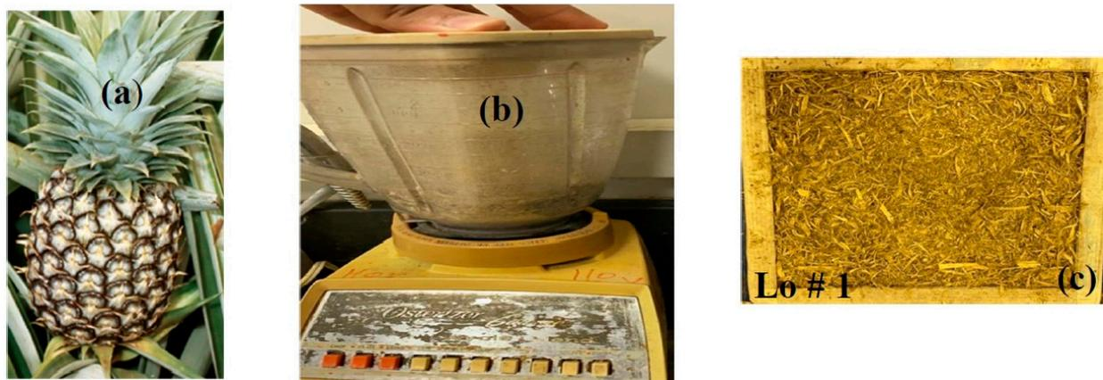
**Figure 1.** Preparation of pineapple leaf fiber; (a) crown leaves, (b) blender used for grinding the crown leaves, and (c) pineapple leaf fiber (PALF) (loose sample # 1).
