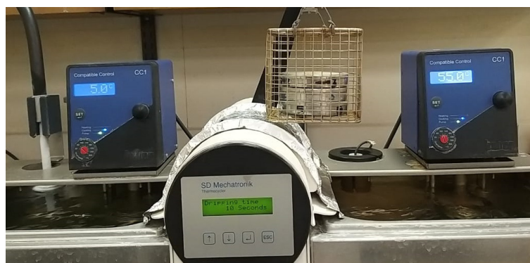
Figure 7. The specimens in the thermocycling unit.
