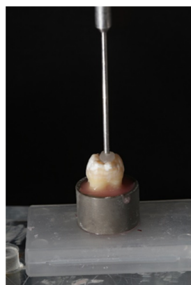
Figure 1. Sample preparation: Teeth were suspended in the center of an aluminum cylinder and mounted 2 mm apical to the cement–enamel junction in polymethyl methacrylate resin.
