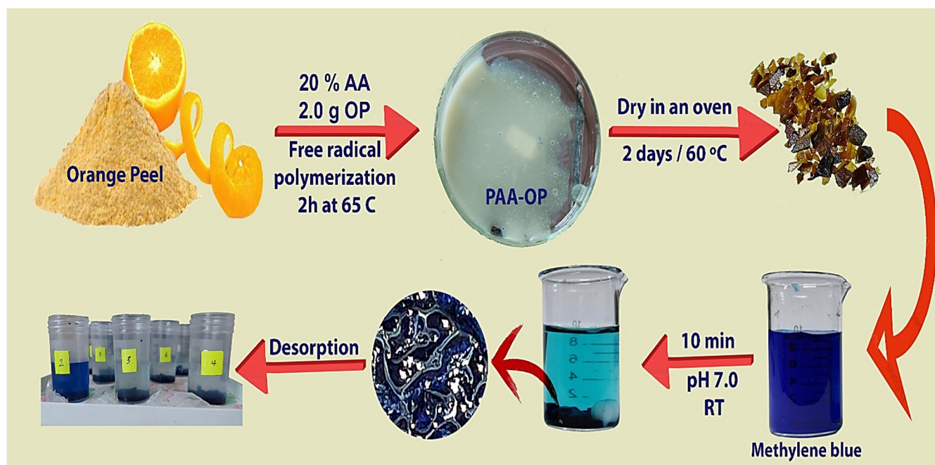
Figure 13. Adsorption and Desorption of MB from Polymer E at different pH (2–9). Experimental conditions were: adsorbents hydrogel dose: 2.0 g in 25 mL for 1 h at RT.
