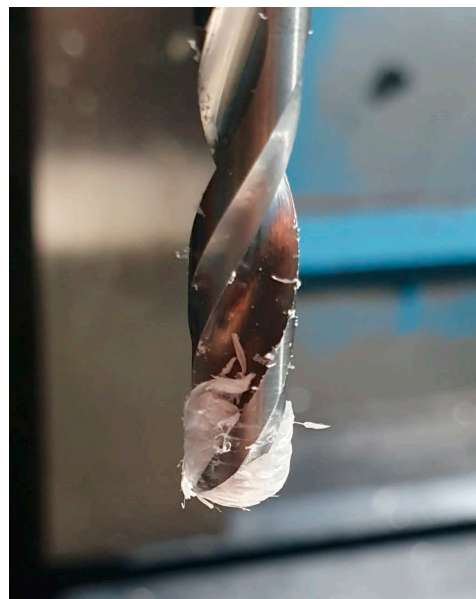
Figure 9. Plug generated at the tip of the bit during the drilling of the UHMWPE composite with the brad and spur geometry.
