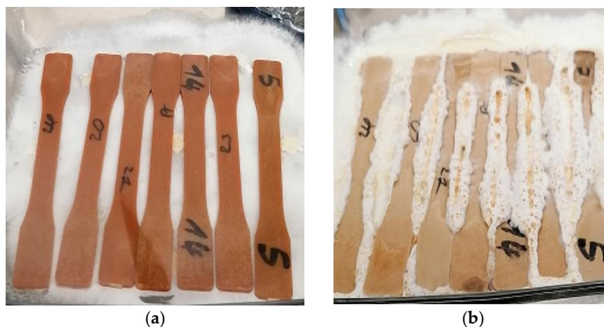
**Figure 3.** Samples exposed at day 1 of exposure (a) and day 30 of exposure (b).
