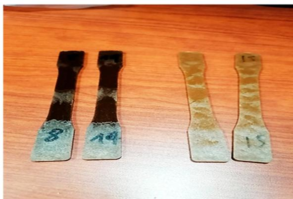
**Figure 2.** ZnO-nontreated tensile test samples (darkest) and ZnO-treated samples.
