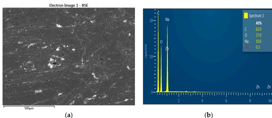
**Figure 9.** (a) ZnO-treated sample's tangential section observed at G 100 $\times$  exposed to *G. trabeum* and (b) EDX analysis.
