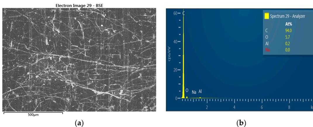
Figure 8. (a) Nontreated sample's tangential section observed at  $G 100\times G$ . *G. trabeum* hyphae are visible (b) EDX analysis.
