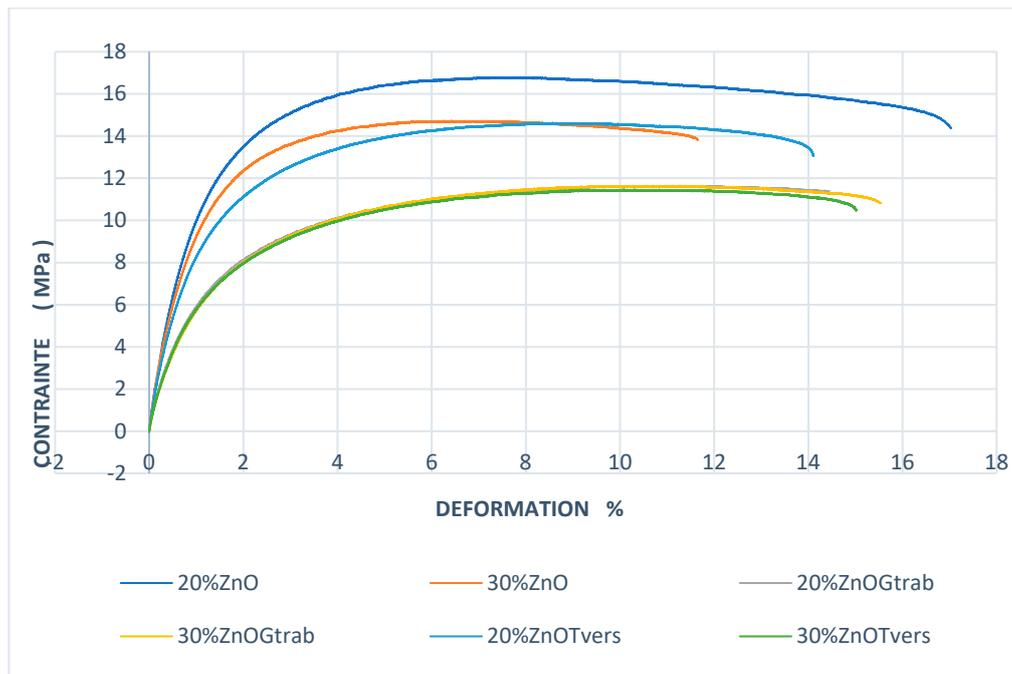
**Figure 6.** Stress-strain behavior of ZnO-treated samples exposed to rot. Legend: 20%ZnO: 20% samples treated with ZnO; 30%ZnO: 30% samples treated with ZnO; 20%ZnOGtrab: 20% samples treated with ZnO and exposed to *G. trabeum*; 30%ZnOGtrab: 30% samples treated with ZnO and exposed to *G. trabeum*; 20%ZnOTvers: 20% samples treated with ZnO and exposed to *T. versicolor*; 30%ZnOTvers: 30% samples treated with ZnO and exposed to *T. versicolor*.
