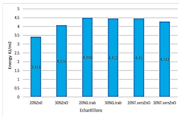
**Figure 4.** Izod impact energy of ZnO-treated HDPE/birch fiber composites exposed and non-exposed to rot. Legend: G.trab: exposed to *Gloephyllum trabeum*; T.vers: exposed to *Trametes versicolor*; ZnO: treated with zinc oxide; 20 and 30%: yellow birch fiber content.
