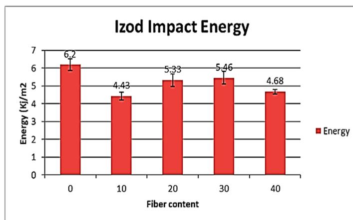
Figure 5. Impact energy of HDPE/yellow birch fiber [6].
