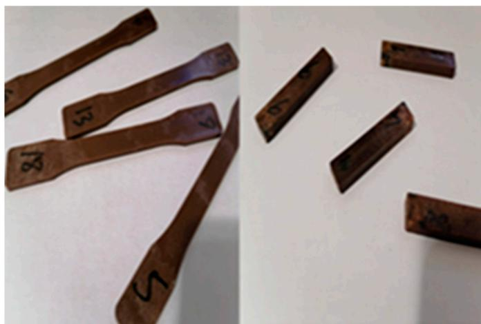
**Figure 1.** Tensile test samples are the largest and Charpy samples the smallest.
