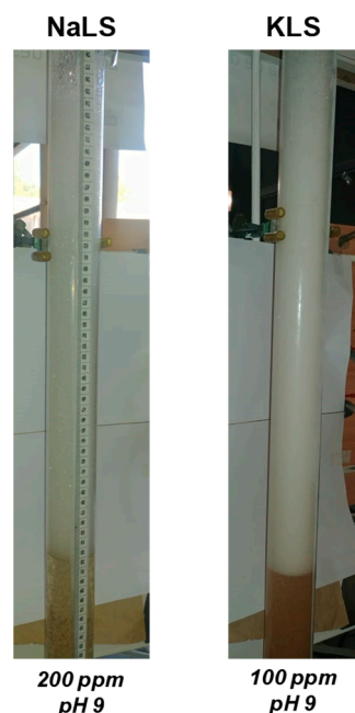
Figure 13. Foams obtained using different lignosulfonates (NaLS and KLS samples).
