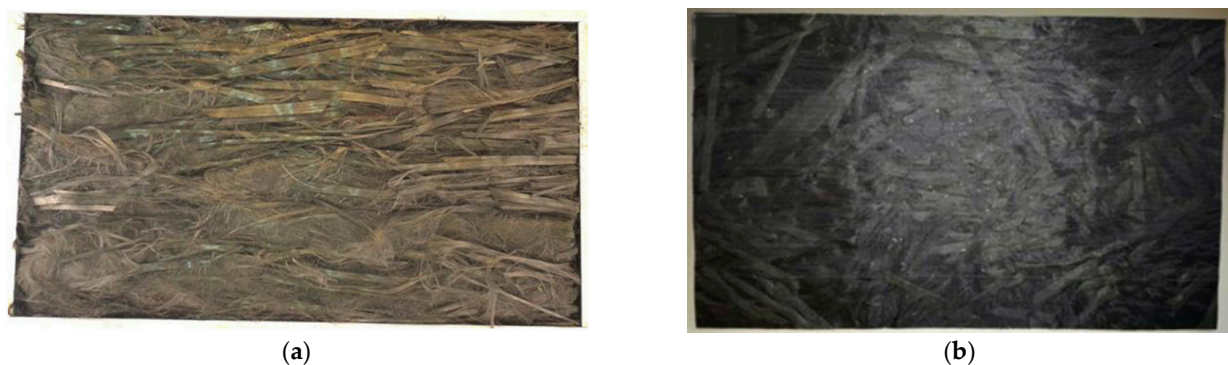
Figure 7. (a) Recycled carbon fibers bundle before brushing resin; (b) rCFRP board [76].
