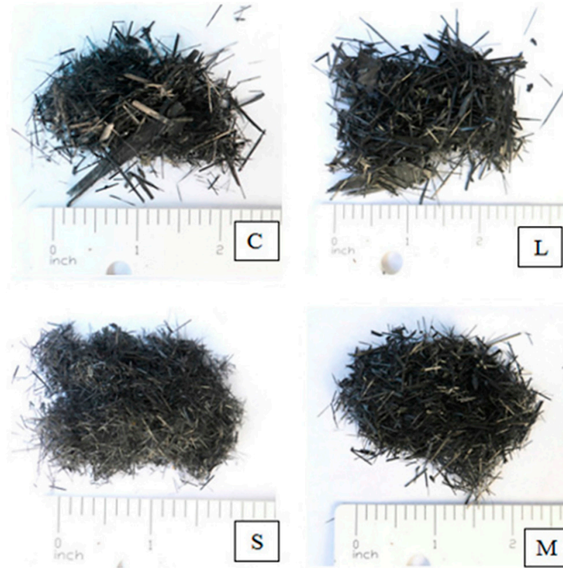
Figure 9. Four different sizes of CFRP were included in the experiment: C-combined, L-large, S-small, and M-medium fraction [120].
