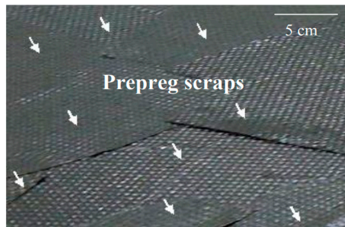
Figure 6. Laminate made from waste prepreg [75].
