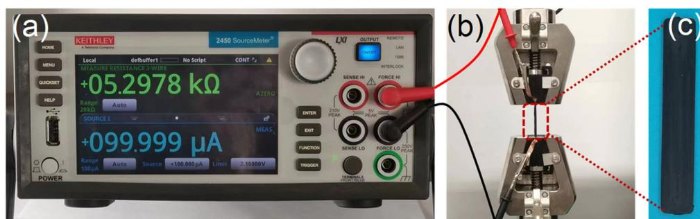
**Figure 1.** The experimental setup for measuring the electro-mechanical properties of CPCs. (a) A sourcemeter was used to measure the resistance change during the mechanical tests. (b) An electro-mechanical testing frame was used to conduct mechanical tests. (c) The strip specimens.
