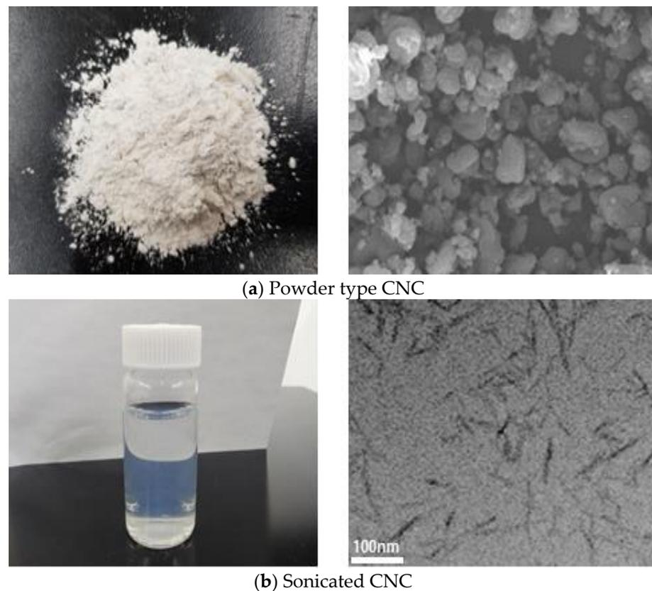
**Figure 2.** CNC shape before and after dispersion.
