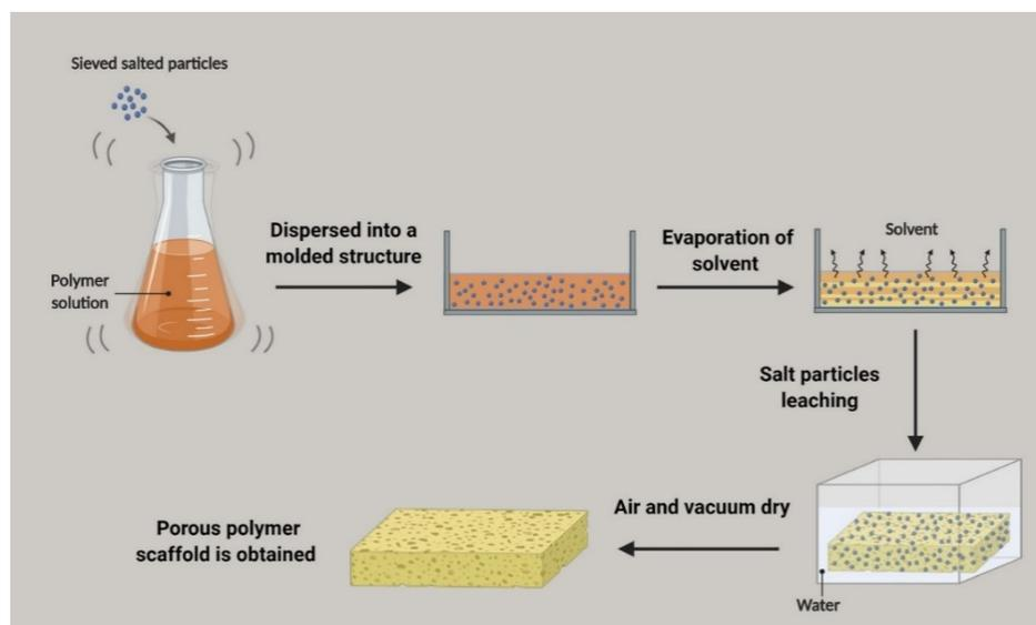
**Figure 8.** Schematic illustration of the solvent casting and particulate leaching technique, [source: [200], redesigned with copyright permission from Elsevier license number: 4724150945567, dated 8 December 2019].
