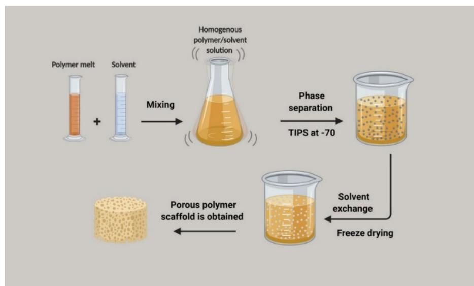
**Figure 6.** Schematic representation of the porous scaffold fabrication process with the Thermally Induced Phase Separation (TIPS), [source: [200], redesigned with copyright permission from Elsevier license number: 4724150945567, dated 8 December 2019].
