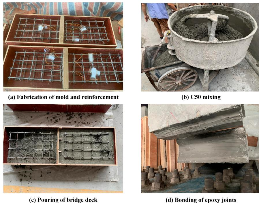
**Figure 5.** Construction process of the specimens: (a) fabrication of mold and reinforcement; (b) C50 mixing; (c) pouring of bridge deck; (d) bonding of epoxy joints.
