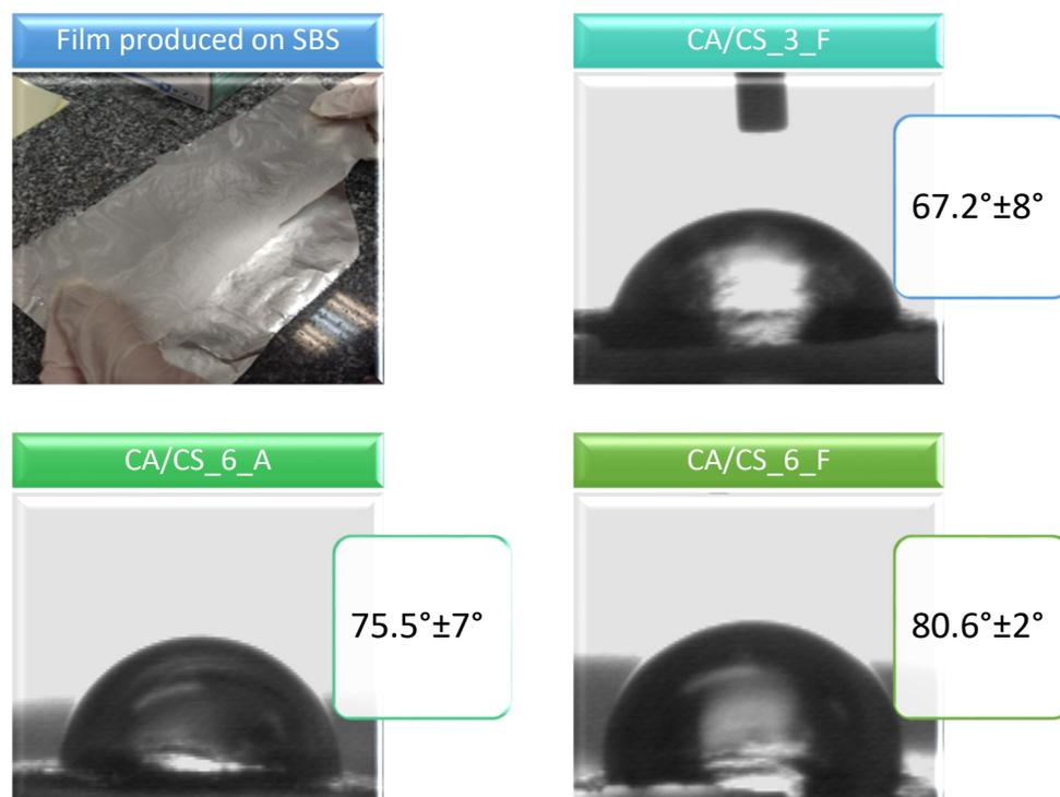
**Figure 2.** Example of CA/CS film produced using solution blow spinning (size after the removal from the collector  $18 \times 5 \text{ cm}^2$ ); the water drops and corresponding contact angles on films' surfaces.
