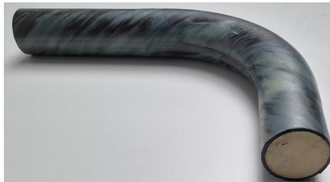
Figure 15. Example of the curved part of polymer composite frame with the following parameters: major radius R = 102.5[\text{mm}] , minor radius r = 17.5[\text{mm}] , width of roving d = 5[\text{mm}] . The non-load-bearing polyurethane frame is visible in the vertical section (light colour of the cross-section).
