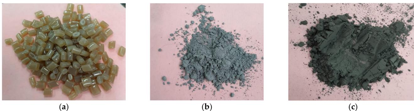
**Figure 1.** (a) Recycled PET granules, (b) Al nanopowder, and (c) Fe nanopowder.
