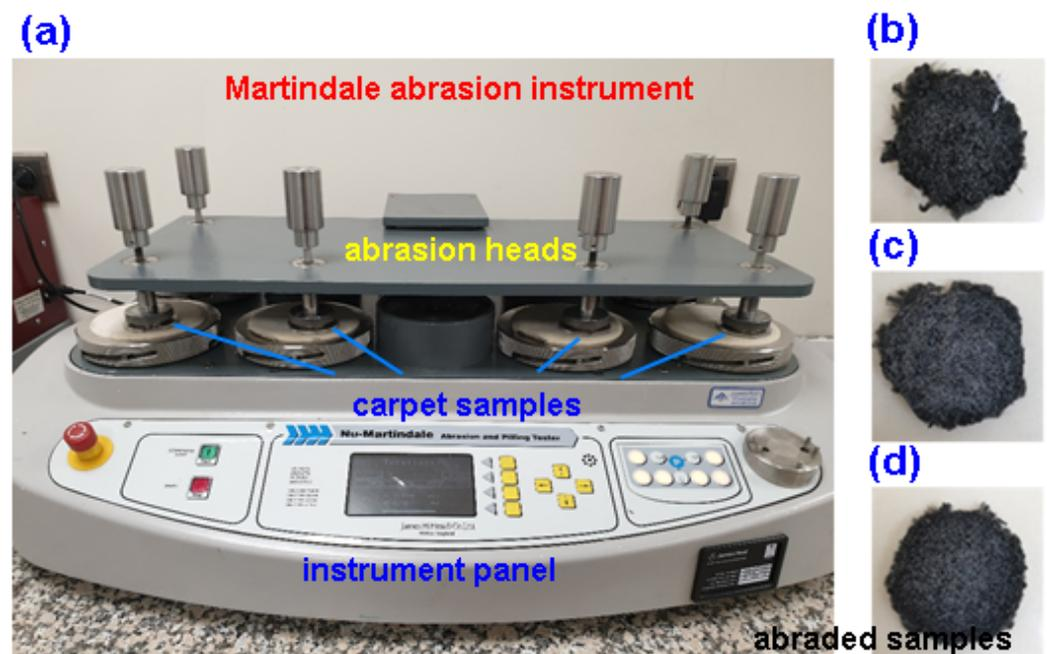
**Figure 5.** (a) Martindale abrasion instrument during testing of carpet structure, (b) image of abraded loose carpet long pile (IPES12), (c) image of abraded dense carpet long pile (2PES12), and (d) image of abraded very dense carpet long pile (3PES12) structure samples (digital photos).
