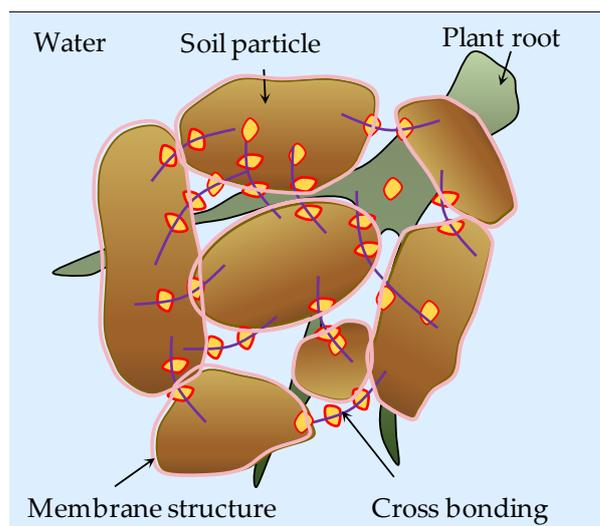
**Figure 3.** Diagram of the interaction mechanism between polymer modifier and soil.
