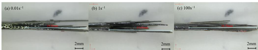
**Figure 15.** Failure morphologies of the sides the  $0^\circ$  specimens of quasi-isotropic-ply laminates at different strain rates.
