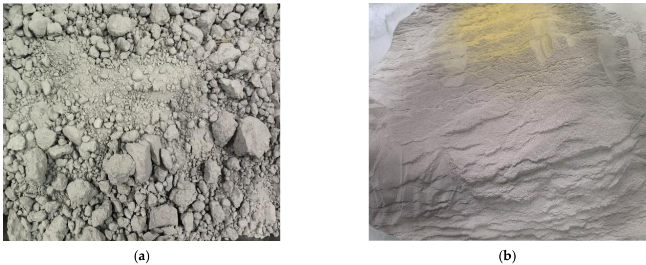
Figure 1. Appearance and morphology of phosphogypsum. (a) Original phosphogypsum; (b) phosphogypsum powder.
