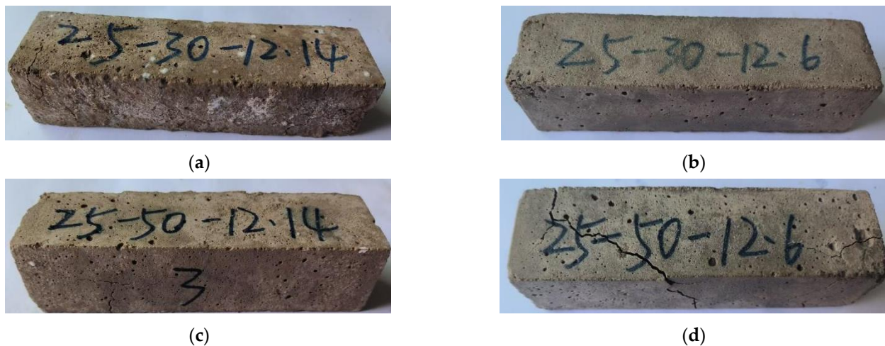
Figure 15. Appearance morphology of mortar specimens with different slag contents after standard curing/water curing for 90 days. (a) R45S30 (S90); (b) R45S30 (W90); (c) R25S50 (S90); (d) R25S50 (W90).
