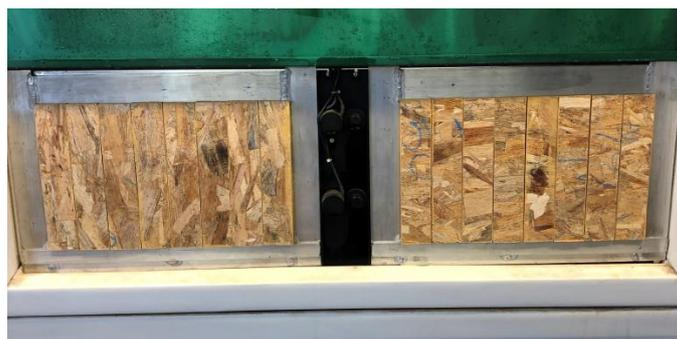
**Figure 3.** Basal wood OSB specimens in artificial aging chamber.
