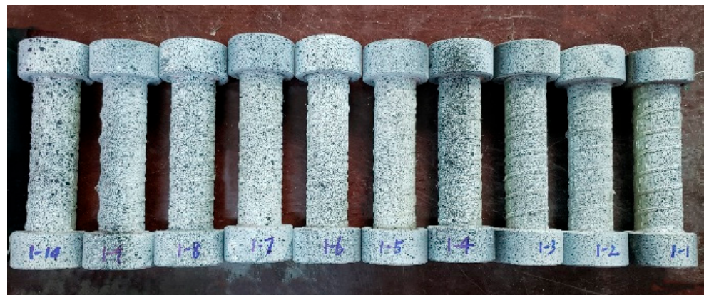
Figure 6. Specimens sprayed with speckles: C1–C10.
