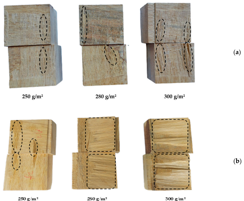
Figure 9. Images of wood failure after the block-shear test of CLT bonded with MF-0 (a) and MF-1 (b) at different glue spreads.
