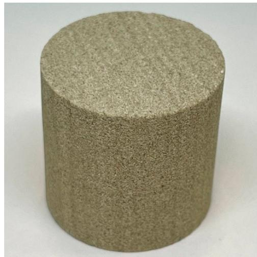
**Figure 1.** A core of the Berea sandstone ("Split rock" type) used for the research.
