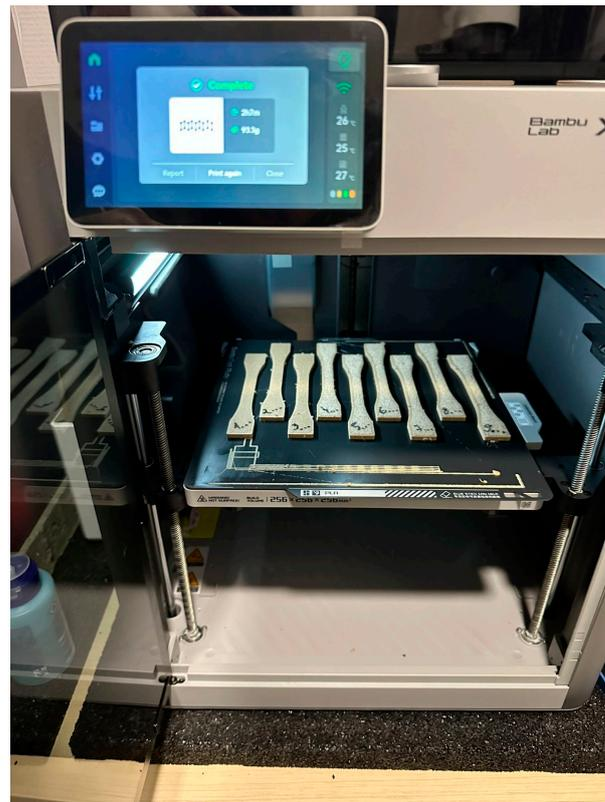
**Figure 3.** The Bambu Lab 3D FDM printer used in the experiments.
