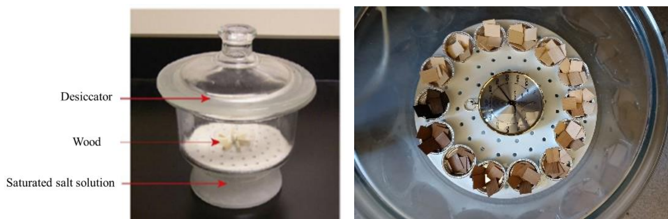
Figure 2. Desiccator used for wood wetting (left). Wood samples are placed from low to high heat treatment temperature (right).
