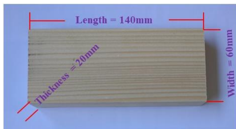
Figure 1. Schematic diagram of wood dimensions for heat treatment.
