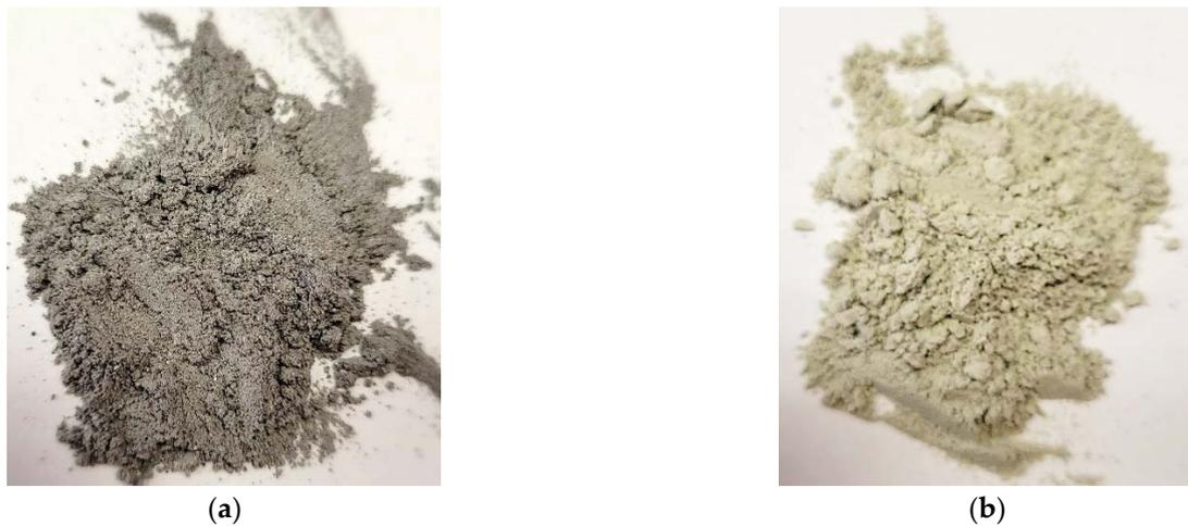
**Figure 1.** The fillers used: (a) Fly ash from the SDPP; (b) Backfill material obtained from the mineral processing waste of the copper-mining plant.
