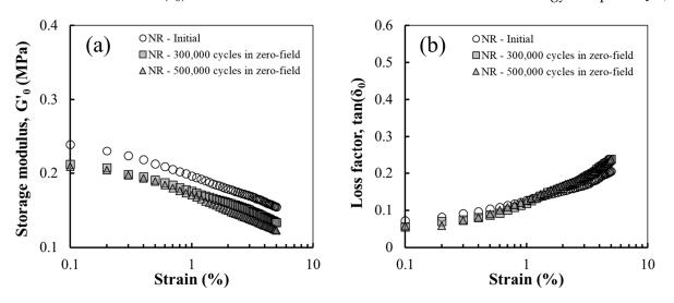
**Figure 3.** (a)  $G'_0$  and (b)  $tan(\delta_0)$  of the NR before and after cyclic shear fatigue.
