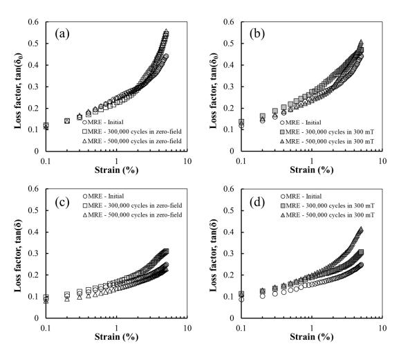
**Figure 5.** Off-state  $tan(\delta_0)$  of the MRE sample before and after cyclic shear fatigue in the (**a**) absence and (**b**) presence of a magnetic field. On-state  $tan(\delta)$  of the MRE sample before and after cyclic shear fatigue in the (**c**) absence and (**d**) presence of magnetic field.
