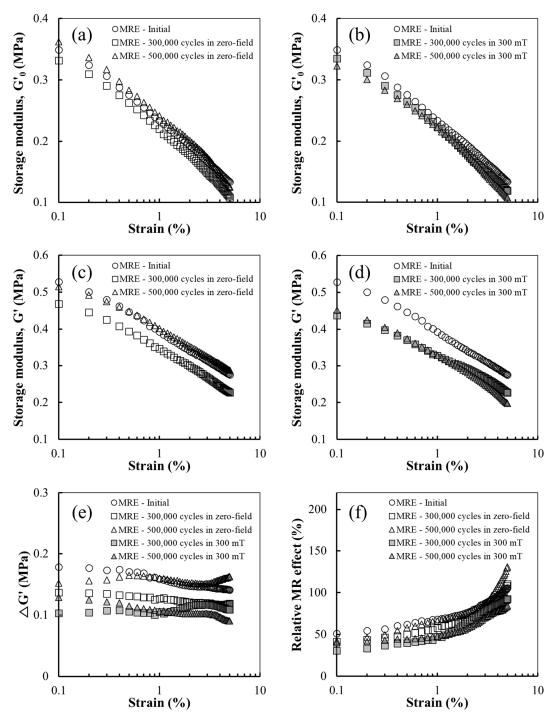
**Figure 4.** Off-state  $G'_0$  of the MRE sample before and after being subjected to cyclic shear fatigue in the (**a**) absence and (**b**) presence of a magnetic field. On-state G' of the MRE sample before and after cyclic shear fatigue in the (**c**) absence and (**d**) presence of magnetic field. (**e**) Absolute and (**f**) relative MR effects of the MRE samples.
