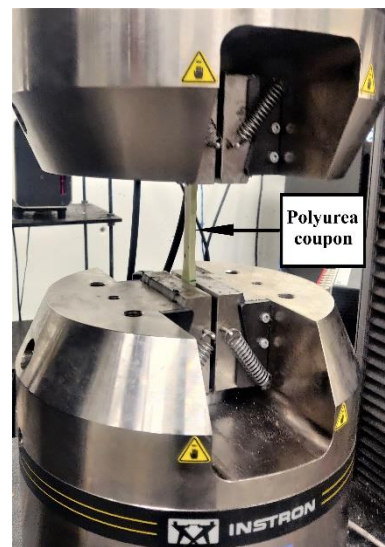
Figure 3. Test Setup featuring a typical die type I coupon specimen installed in the Instron UTM.
