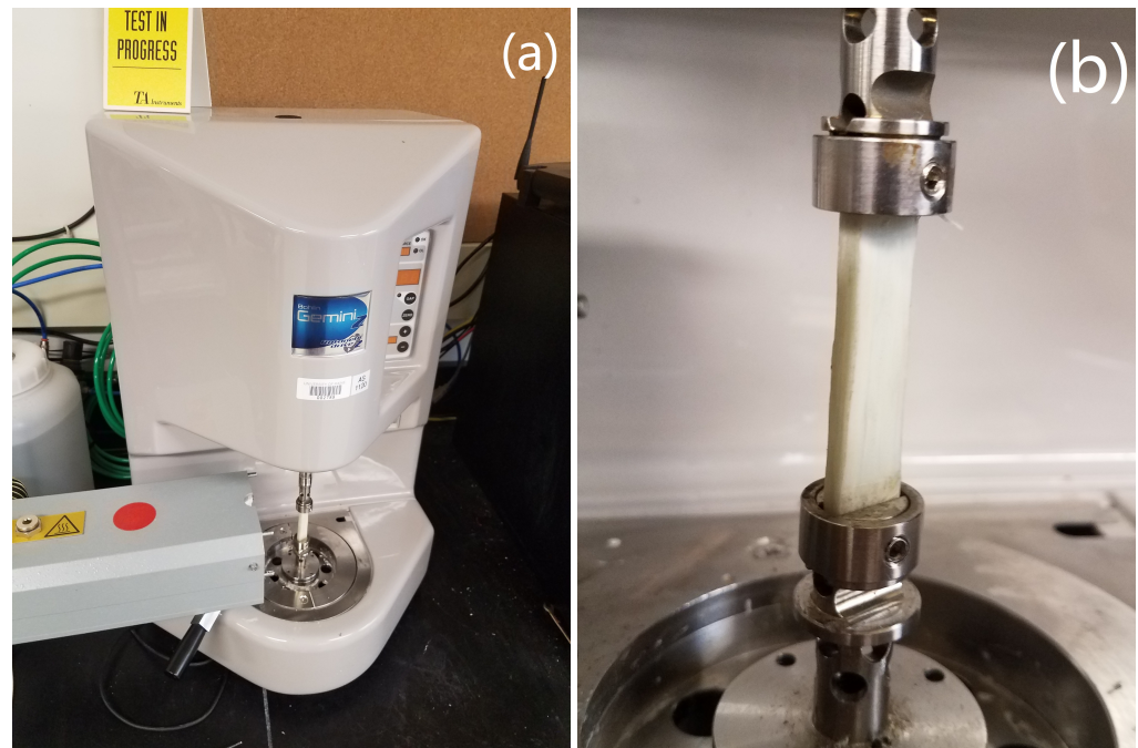
Figure 3. Photos of the torsional rheometer experimental setup. (a) Bohlin rheometer with ETC; (b) 10 mm × 4 mm × 35 mm specimen installed in fixture clamps.
