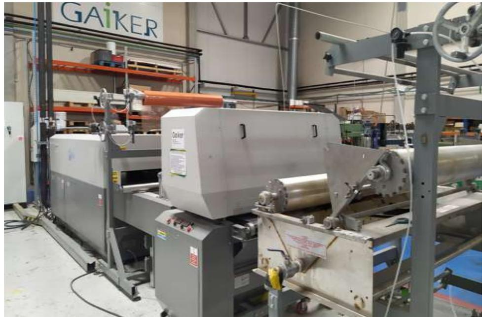
**Figure 2.** Reliant Powerbond double-belt laminating equipment model.
