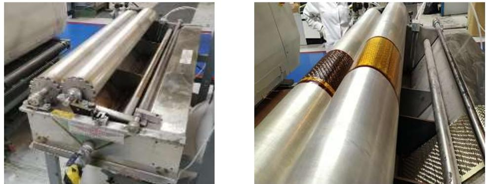
**Figure 1.** Phoenix PI 6000 model prepreg equipment.
