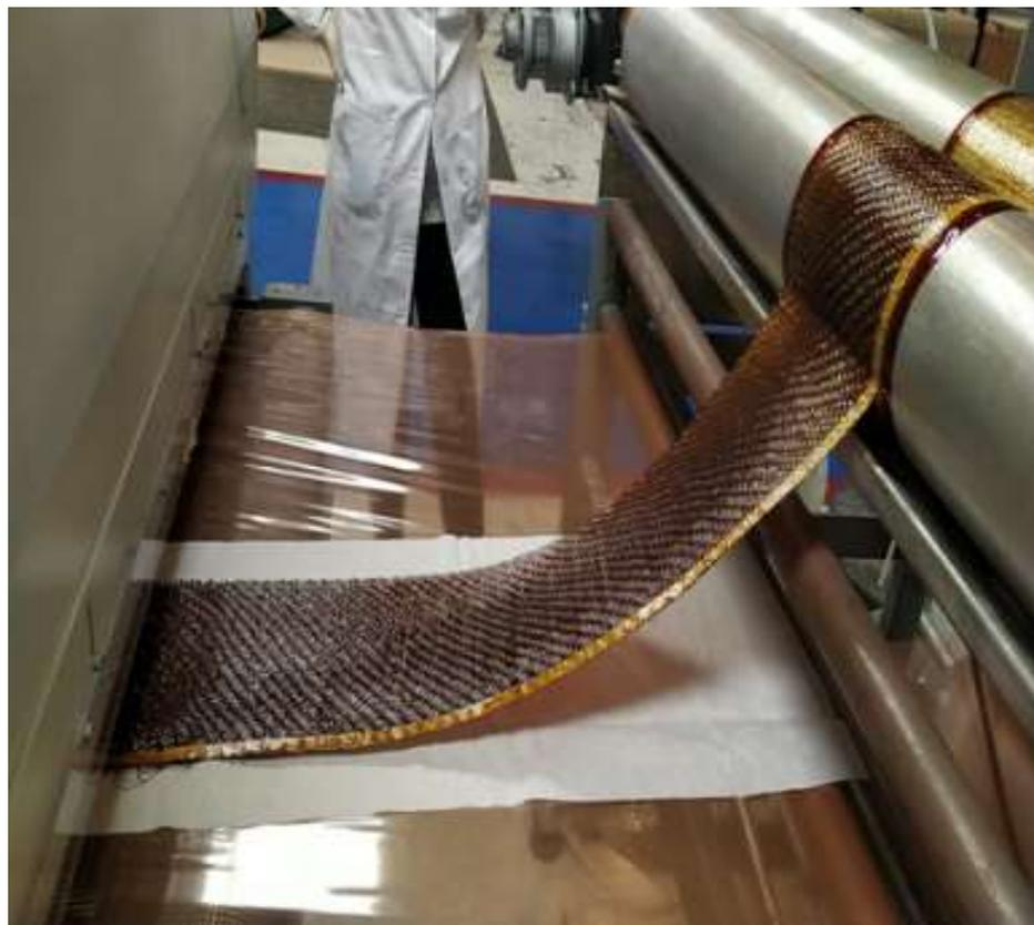
**Figure 3.** Impregnation of the fibre and subsequent laying on siliconized paper.
