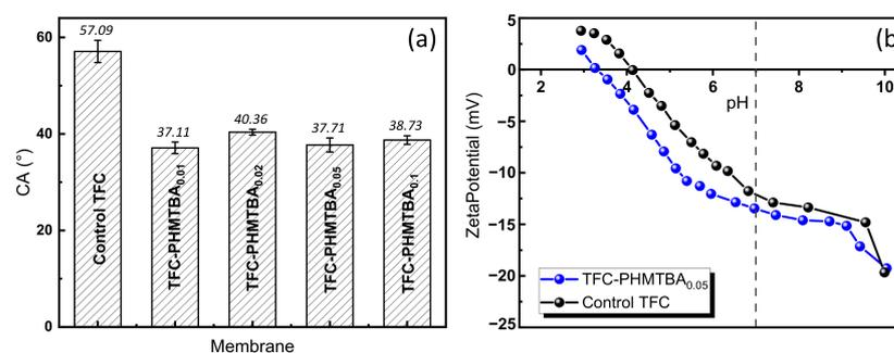
**Figure 6.** (a) WCA of unmodified and PHMTBA–modified membranes and (b) zeta potential at different pH values of control TFC and PA–PHMTBA<sub>0.05</sub> membranes.
