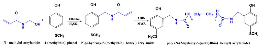
**Figure 1.** The synthesis route of self-polymer PHMTB.
