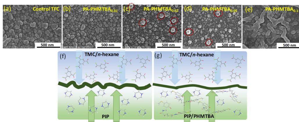
**Figure 5.** (a–e) SEM surface images and (f,g) schematic diagrams of the interfacial diffusion process of unmodified and PHMTBA-modified TFC membranes. (The red coils in (c,d) represented the particle-like structure).
