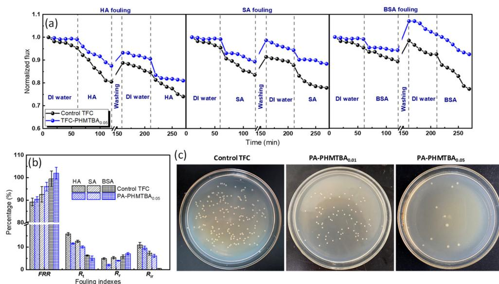
**Figure 9.** Anti-fouling properties of the as-prepared TFC membrane. (a) Normalized fluxes with various pollutants filtration, (b) fouling indexes, and (c) images of Petri dishes of the unmodified and PHMTBA-modified membranes.
