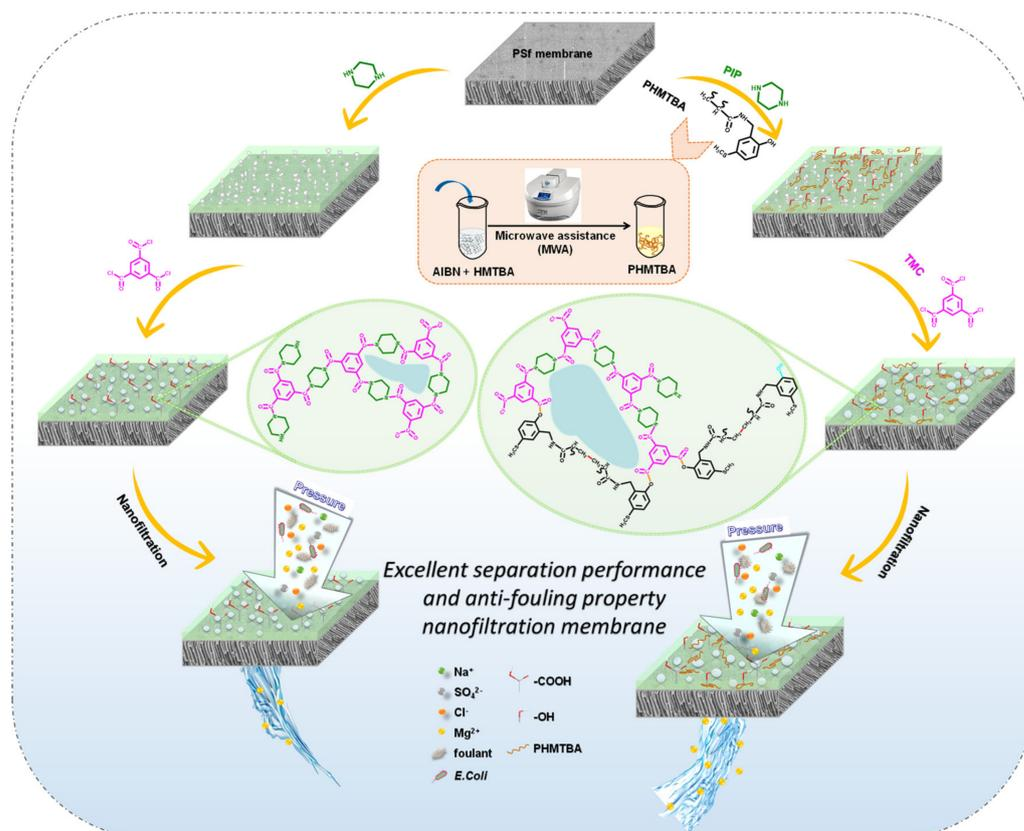
**Figure 2.** The schematic diagram of a fabrication process of unmodified and PHMTBA-modified TFC membranes.
