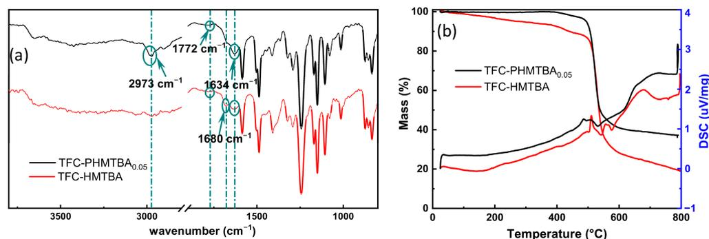
**Figure 3.** (a) FTIR spectra and (b) TG curve of PA-PHMTBA and PA-HMTBA membranes.
