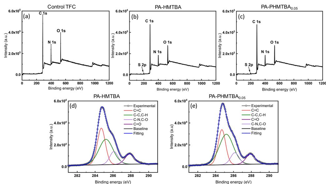
**Figure 4.** XPS assessment of as-fabricated membranes. XPS spectra of (a) control TFC membranes, (b) PA-HMTBA membranes, and (c) PA-PHMTBA membranes; C1s survey spectra of (d) PA-HMTBA and (e) PA-PHMTBA membranes.
