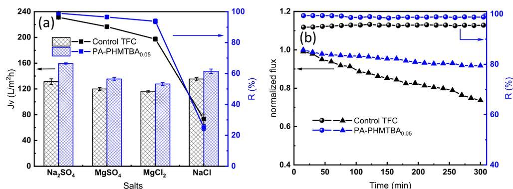
**Figure 8.** (a) Selectivity for different inorganic salt solutions and (b) stability of the control TFC membrane and the PA-PHMTBA<sub>0.05</sub> membrane.
