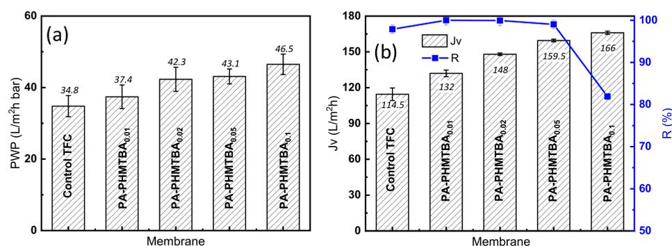
**Figure 7.** (a) Permeance and (b) selectivity of prepared TFC membranes.
