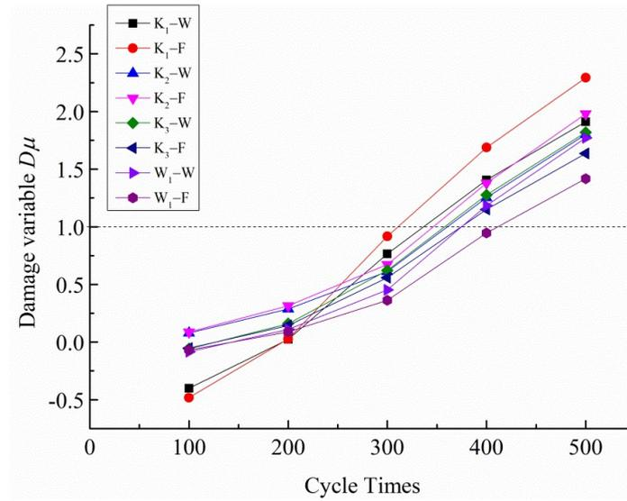
Figure 8. Curves of the damage variable  $Du$  and cycle number.
