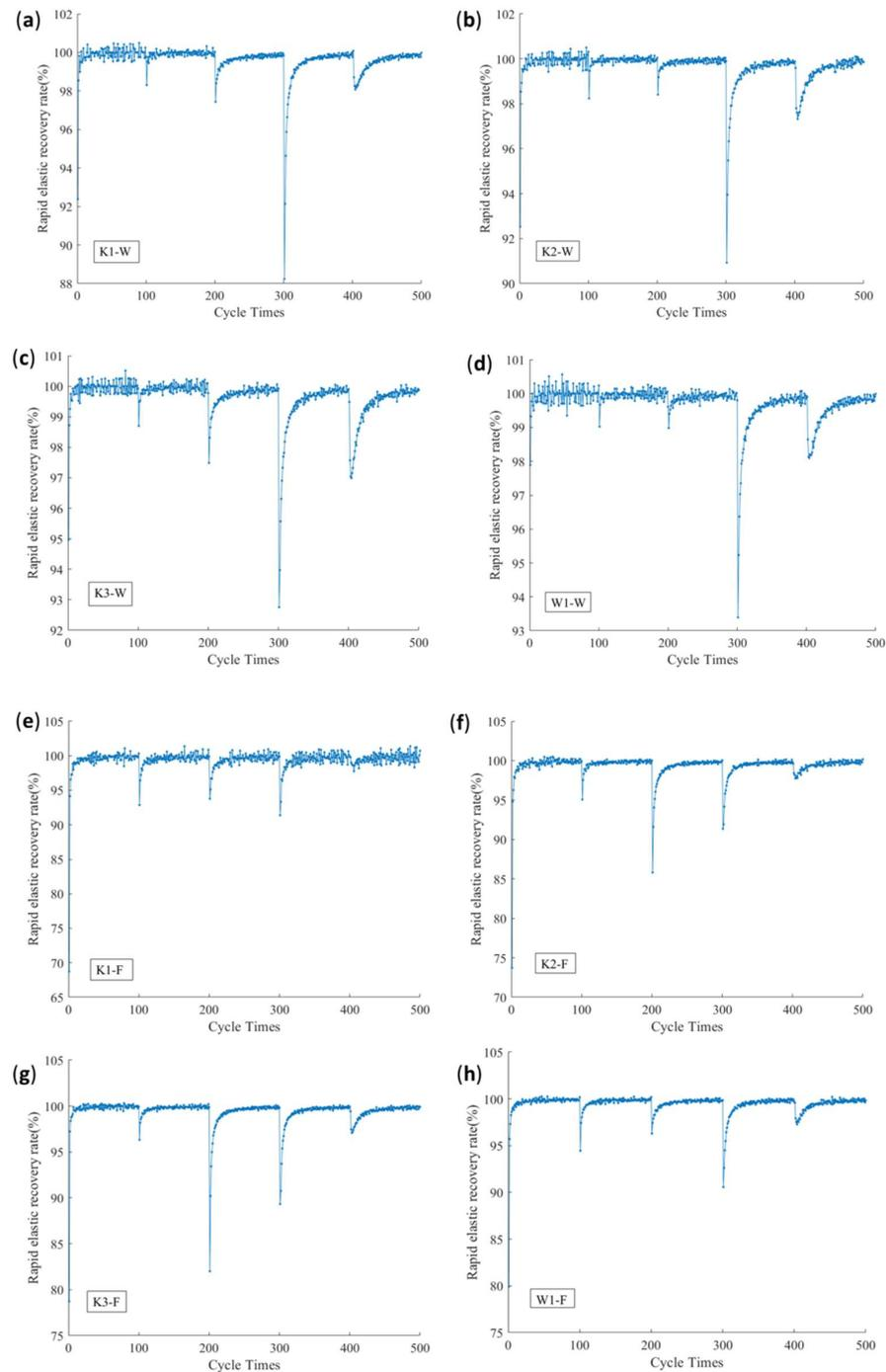
**Figure 7.** Variation curves of the rapid elastic recovery rate with stress. (a–d) Rapid elastic recovery rate of the warp direction of  $K_1$ ,  $K_2$ ,  $K_3$ , and  $W_1$ . (e–h) Rapid elastic recovery rate of the fill direction of  $K_1$ ,  $K_2$ ,  $K_3$ , and  $W_1$ .
