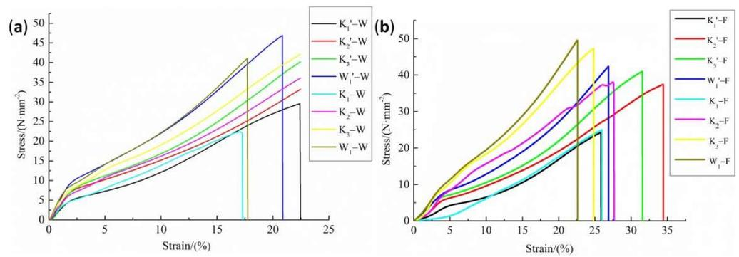
**Figure 1.** Fracture stress–strain curves of the tested specimens. (a) Warp direction; (b) fill direction.
