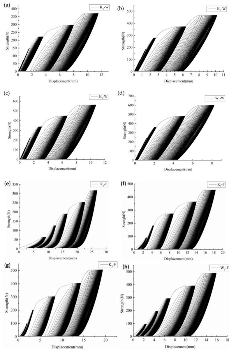
**Figure 2.** Stress–strain curves of the tested specimens under multistage cyclic loading and unloading. (a–d) Warp direction of  $K_1$ ,  $K_2$ ,  $K_3$ , and  $W_1$ ; (e–h) fill direction of  $K_1$ ,  $K_2$ ,  $K_3$ , and  $W_1$ .
