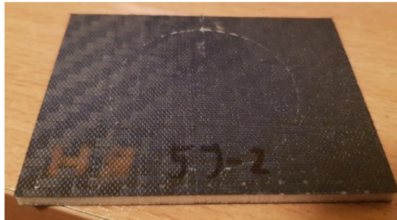
Figure 10. Herex 55 core specimen with face cracking on the side opposite to the impact.
