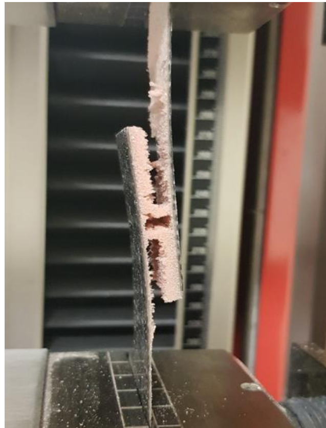
Figure 17. Test sample destroyed in the grip of a Herex core testing machine.
