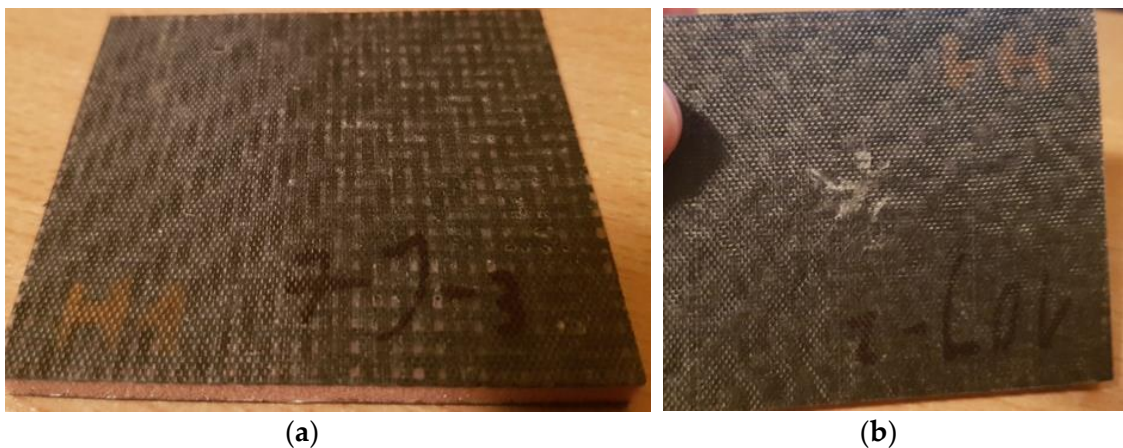
Figure 11. Opposite impact side of composite with Herex 90 core: (a) 7 J energy and (b) 10 J energy.
