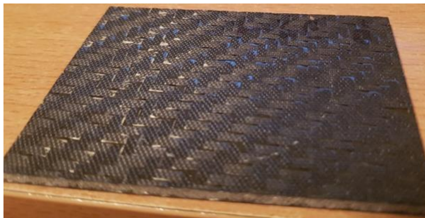
Figure 8. Composite with Airex foam core on the opposite side of the impact—energy 3 J.
