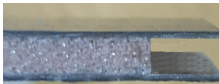
Figure 18. Modified end section of the sample for the tensile strength tests.
