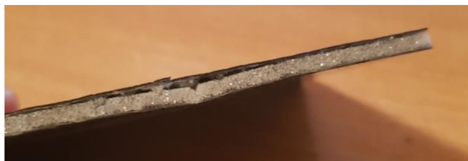
Figure 12. Separated core and face in the composite with Airex core.
