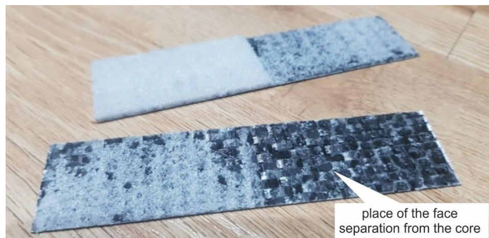
Figure 16. Destroyed sample during an adhesion test between the core and the faces of Airex core composite.
