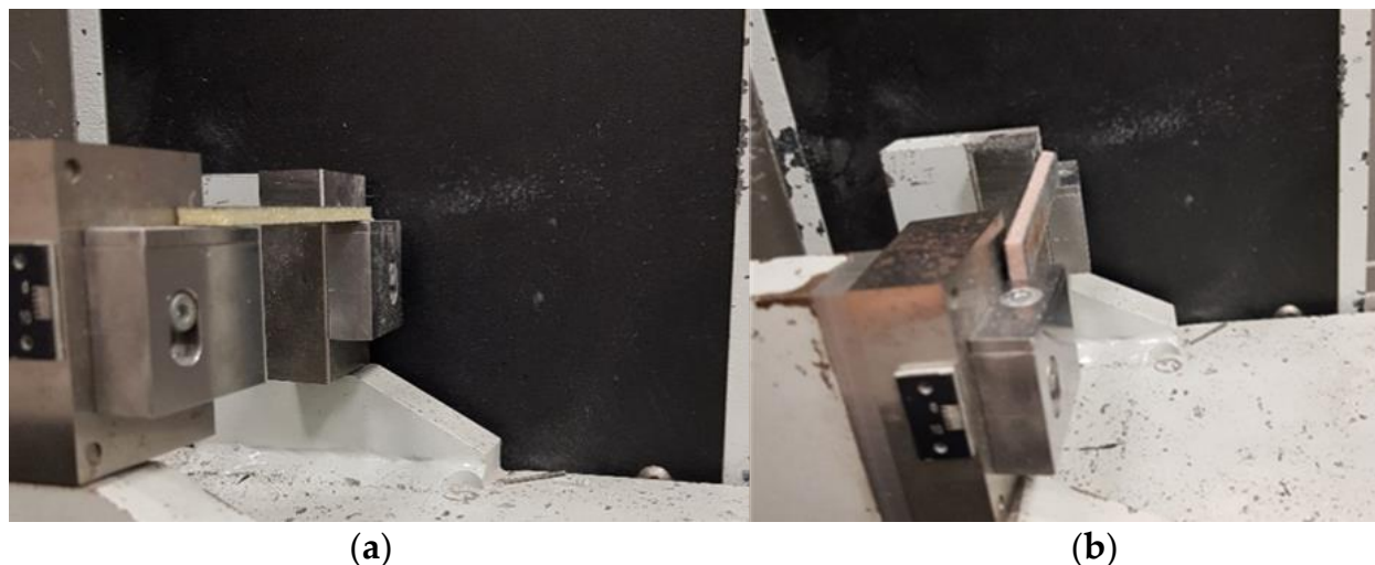
Figure 2. Sample placed for impact testing under: (a) edgewise loading and (b) flatwise loading.
