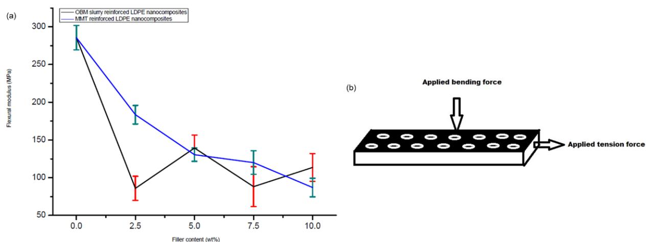
**Figure 14.** (a) Comparison of modulus of elasticity in bending of neat LDPE, LDPE/MMT and LDPE/OBM slurry nanocomposites; (b) a schematic illustration of applied force in tension and bending test and the distribution of MMT and OBM slurry nanoplatelets through the sample.
