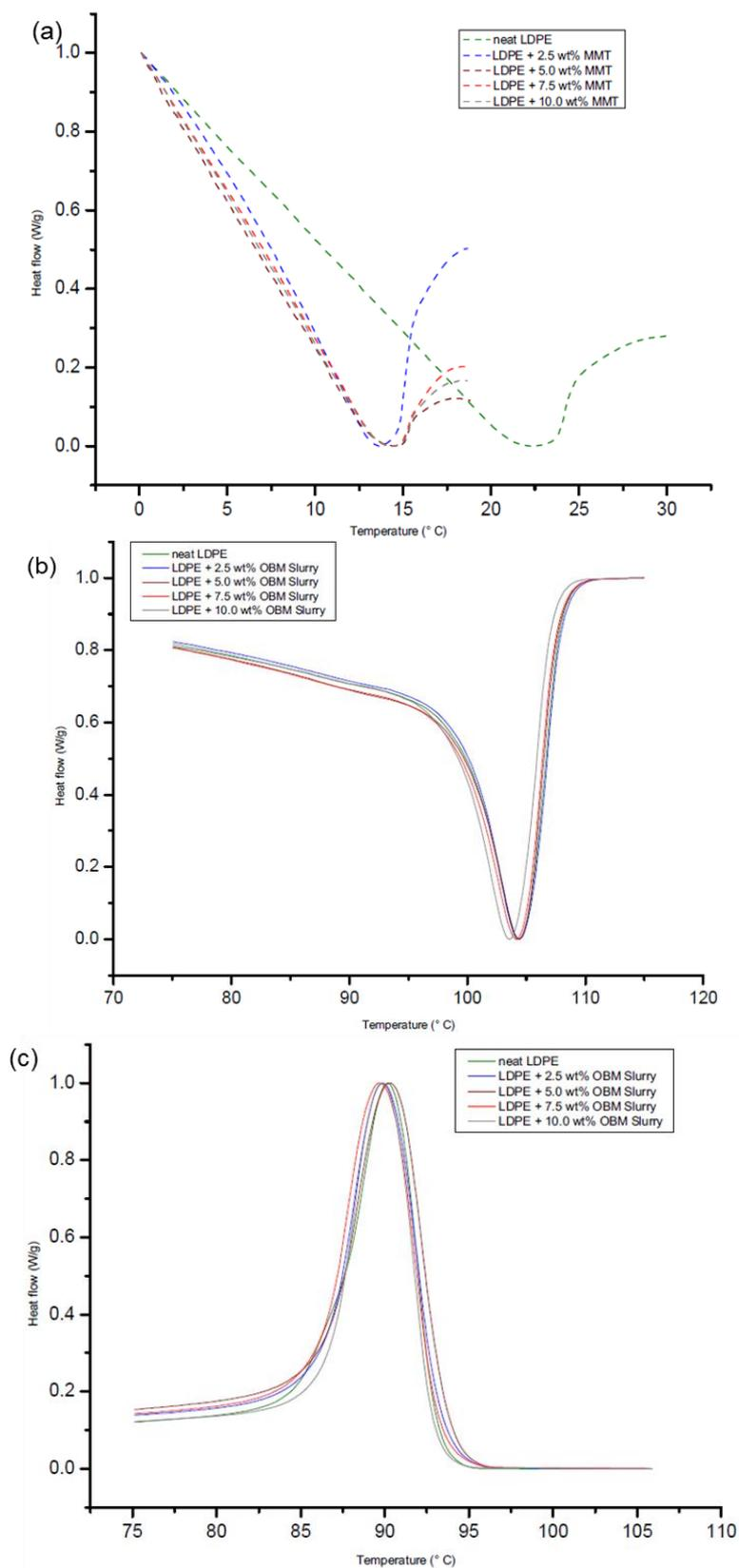
**Figure 15.** DSC thermograms of LDPE and LDPE/MMT nanocomposites at (a) glass transition temperature (T<sub>g</sub>); and LDPE and LDPE/OBM slurry nanocomposites at (b) melting temperature (T<sub>m</sub>) and (c) crystallisation temperature (T<sub>c</sub>).
