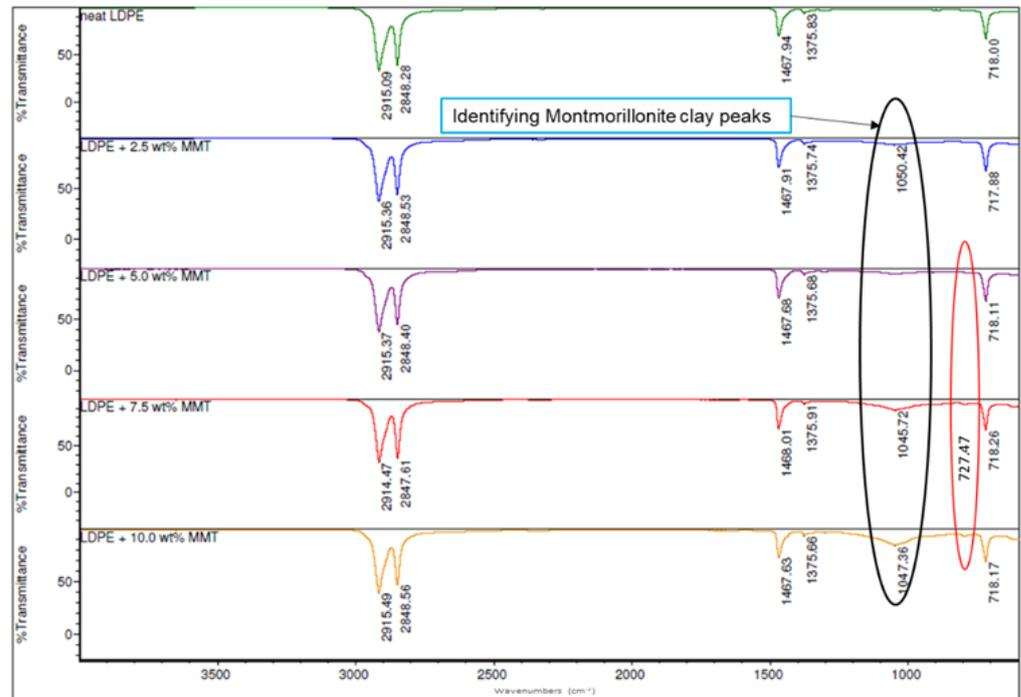
Figure 6. Comparison of ATR-FTIR spectra of LDPE and LDPE/MMT nanocomposites.
