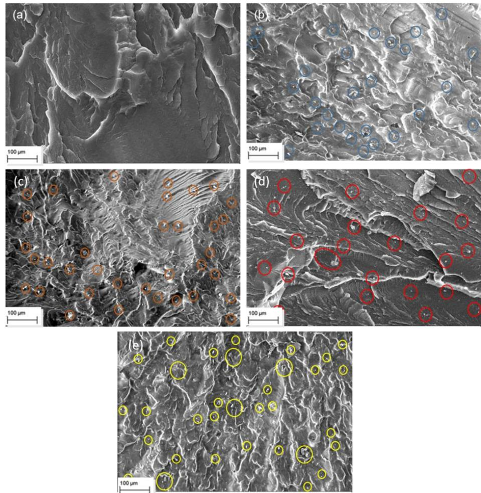
**Figure 4.** SEM images of (a) neat LDPE; (b) LDPE with 2.5 wt% OBM slurry; (c) LDPE with 5 wt% OBM slurry; (d) LDPE with 7.5 wt% OBM slurry and (e) LDPE with 10 wt% OBM slurry.
