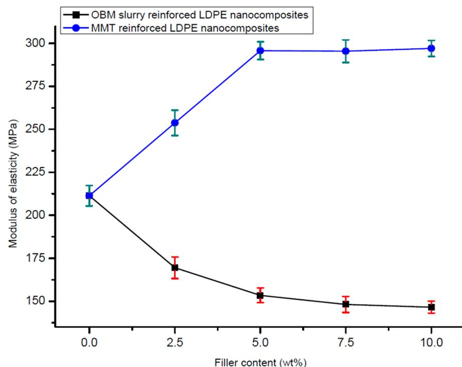
**Figure 10.** Comparison of modulus of elasticity in tension of neat LDPE, LDPE/MMT and LDPE/OBM slurry nanocomposites.
