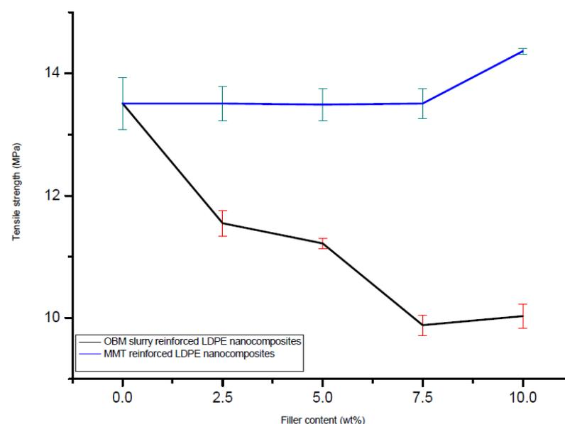
**Figure 9.** Comparison of tensile strength between LDPE/MMT and LDPE/OBM slurry nanocomposites considering tensile strength of neat LDPE as a baseline.
