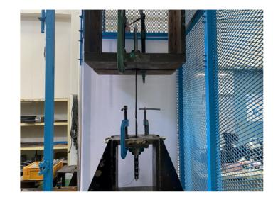
Figure 4. Single-anchorage system tensile test method.
