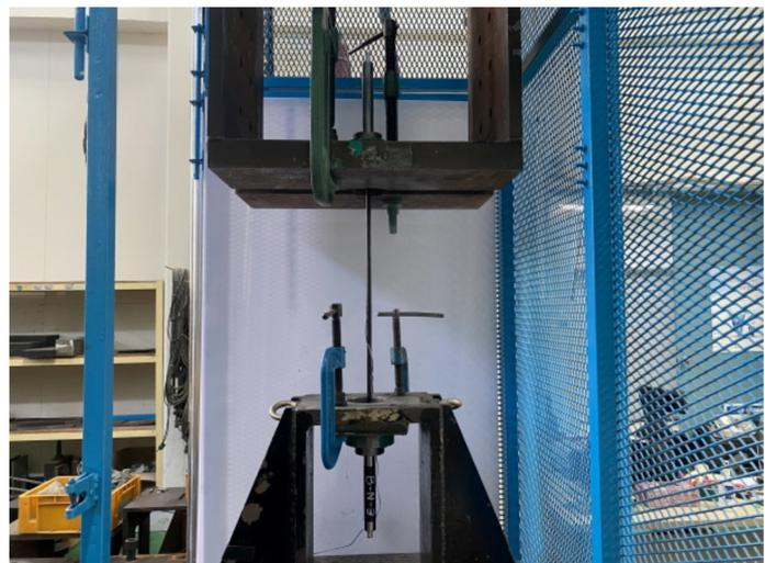
**Figure 4.** Single-anchorage system tensile test method.
