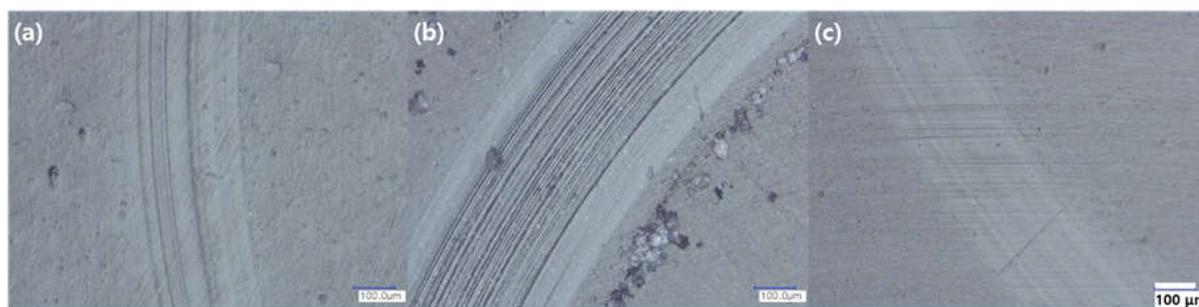
**Figure 7.** Optical micrographs of worn surfaces of (a) DH-10, (b) DR-10, and (c) S05-10 under friction condition (load: 10 N, sliding speed: 400 RPM, duration: 10 min).
